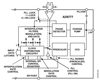
Figure 45. PLL and Clock Circuitry with PLL Enabled
