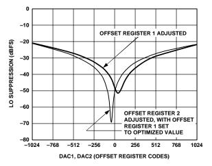
Figure 42. Offset Adjust Control, Effect on LO Suppression
