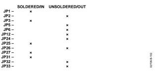
Figure 102. Test Configuration for AD9777 in One-Port Mode with PLL Enabled, Signal Generator Frequency = One-Half Interleaved Input Data Rate, ONEPORTCLK = Interleaved Input Data Rate, DAC Output Data Rate = Signal Generator Frequency × Interpolation Rate
