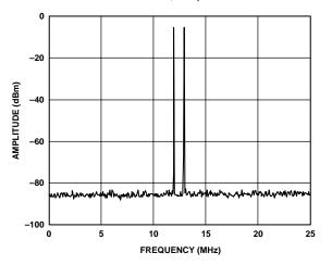
Figure 29. Two-Tone IMD Performance,  $f_{OUT} = 10$  MHz,  $f_{DATA} = 50$  MSPS, Interpolation =  $8 \times$
