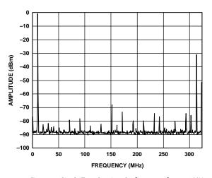
Figure 28. Single-Tone Spurious Performance,  $f_{OUT} = 10$  MHz,  $f_{DATA} = 80$  MSPS, Interpolation =  $4 \times$
