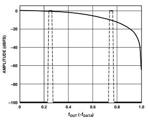
Figure 61. No Interpolation, Modulation =  $f_{DAC}/4$
