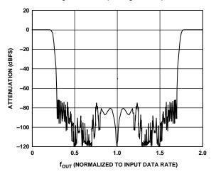
Figure 3. 4× Interpolating Filter Response
