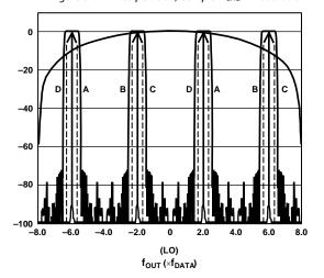
Figure 85. 8× Interpolation, Complex  $f_{DAC}/4$  Modulation
