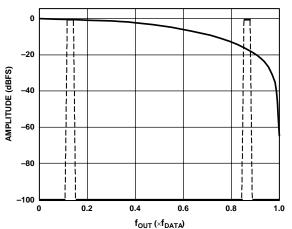
Figure 62. No Interpolation, Modulation =  $f_{DAC}/8$
