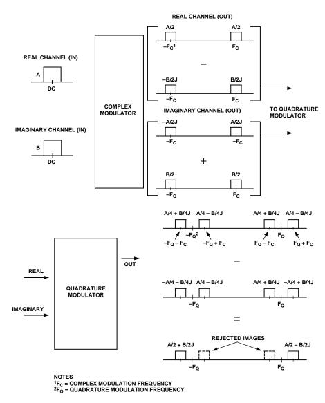
Figure 79. Two-Stage Upconversion and Resulting Image Rejection
