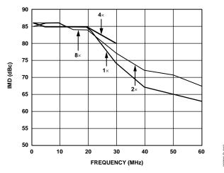
Figure 18. Third-Order IMD Products vs. Two-Tone  $f_{OUT}$  and Interpolation Rate,  $1 \times f_{DATA} = 160$  MSPS,  $2 \times f_{DATA} = 160$  MSPS,  $4 \times f_{DATA} = 80$  MSPS,  $8 \times f_{DATA} = 50$  MSPS
