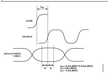
Figure 55. Timing Requirements in Two-Port Input Mode, with PLL Disabled
