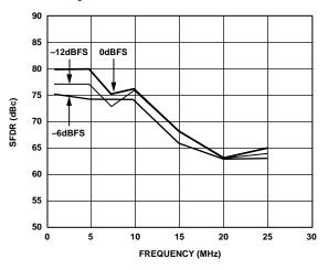
Figure 8. Out-of-Band SFDR vs.  $f_{OUT} @ f_{DATA} = 65 \text{ MSPS}$
