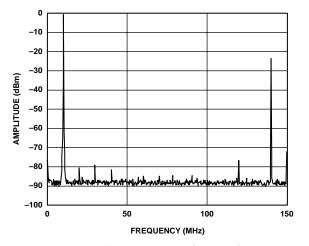
Figure 24. Single-Tone Spurious Performance,  $f_{OUT} = 10$  MHz,  $f_{DATA} = 150$  MSPS, No Interpolation
