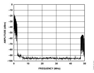
Figure 89. AD9777, Real DAC Output of Complex Input Signal Near Baseband (Positive Frequencies Only), Interpolation =  $4 \times$ , No Modulation in AD9777
