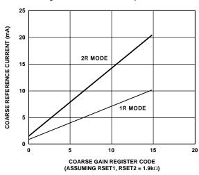
Figure 39. Coarse Gain Effect on IFULLSCALE
