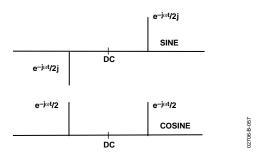
Figure 57. Real and Imaginary Components of Sinusoidal and Cosinusoidal Waveforms
