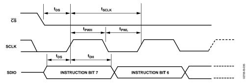
Figure 35. Timing Diagram for Register Write to AD9777
