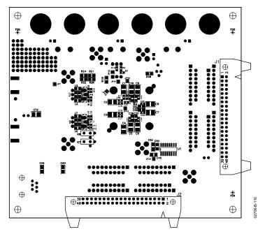
Figure 110. AD9777 Evaluation Board Components, Bottom Side
