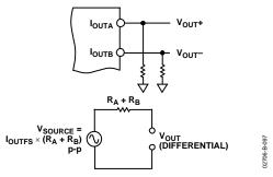
Figure 97. DAC Output Equivalent Circuit
