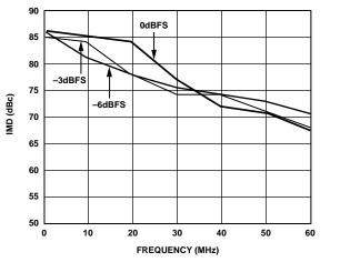
Figure 17. Third-Order IMD Products vs. Two-Tone f<sub>OUT</sub> @ f<sub>DATA</sub> = 160 MSPS
