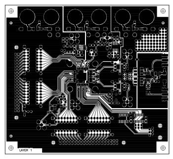
Figure 111. AD9777 Evaluation Board Layout, Layer One (Top)
