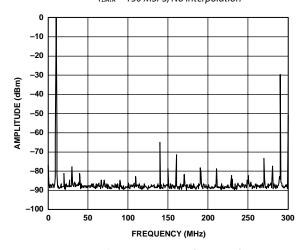
Figure 26. Single-Tone Spurious Performance,  $f_{\text{OUT}} = 10$  MHz,  $f_{\text{DATA}} = 150$  MSPS, Interpolation =  $2 \times$
