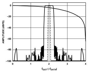
Figure 72. 8x Interpolation, Modulation =  $f_{DAC}/2$
