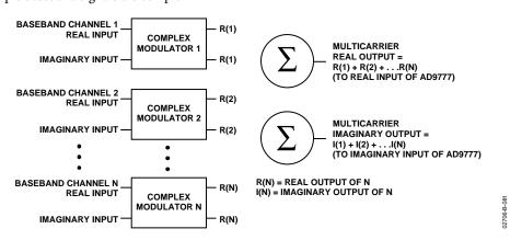
Figure 81. Synthesis of Multicarrier Complex Signal
