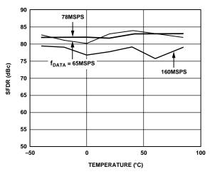
Figure 23. SFDR vs. Temperature @  $f_{OUT} = f_{DATA}/11$
