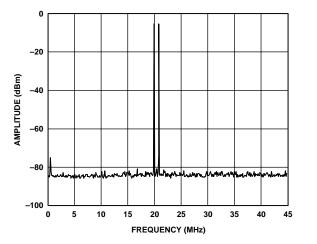
Figure 27. Two-Tone IMD Performance,  $f_{DATA} = 90$  MSPS, Interpolation =  $4 \times$
