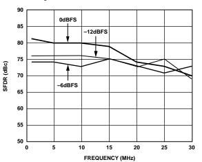
Figure 11. Out-of-Band SFDR vs.  $f_{OUT} @ f_{DATA} = 78 \text{ MSPS}$
