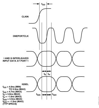
Figure 56. Timing Requirements in One-Port Input Mode, with PLL Disabled
