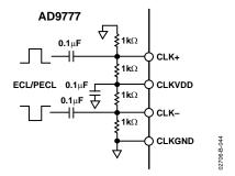
Figure 44. Differential Clock Driving Clock Inputs
