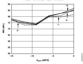
Figure 19. Third-Order IMD Products vs. Two-Tone  $A_{OUT}$  and Interpolation Rate,  $f_{DATA} = 50$  MSPS in All Cases,  $1 \times f_{DAC} = 50$  MSPS,  $2 \times f_{DAC} = 100$  MSPS,  $4 \times f_{DAC} = 200$  MSPS,  $8 \times f_{DAC} = 400$  MSPS
