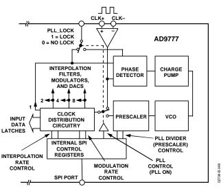
Figure 46. PLL and Clock Circuitry with PLL Disabled
