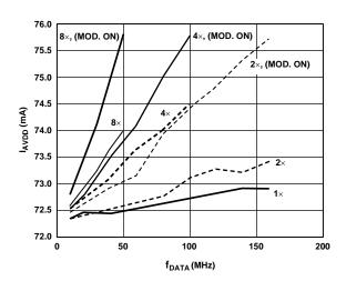
Figure 50. IAVDD vs. f<sub>DATA</sub> vs. Interpolation Rate, PLL Disabled
