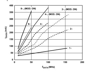
Figure 49. IDVDD vs. fDATA vs. Interpolation Rate, PLL Disabled
