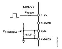
Figure 43. Single-Ended Clock Driving Clock Inputs
