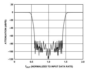
Figure 2. 2× Interpolating Filter Response
