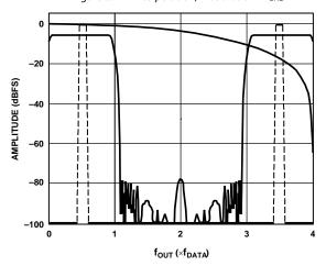
Figure 70. 4x Interpolation,  $Modulation = f_{DAC}/8$
