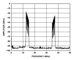
Figure 91. AD9777, Real DAC Output of Complex Input Signal Near Baseband (Positive Frequencies Only), Interpolation =  $4 \times$ , Complex Modulation in AD9777 =  $+ f_{DAC}/4$
