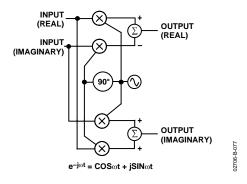
Figure 77. Implementation of a Complex Modulator
