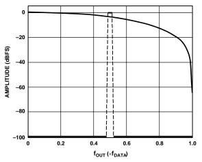
Figure 60. No Interpolation, Modulation =  $f_{DAC}/2$
