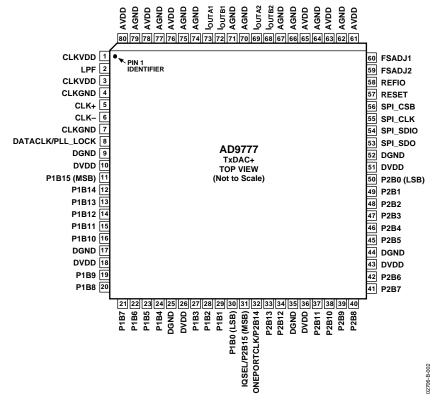
Figure 5. Pin Configuration
