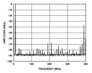
Figure 30. Single-Tone Spurious Performance,  $f_{\text{OUT}} = 10$  MHz,  $f_{\text{DATA}} = 50$  MSPS, Interpolation =  $8 \times$
