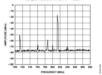
Figure 96. AD9777 Complex Output from Figure 95, Now Quadrature Modulated by AD8345 (LO = 800 MHz)
