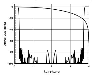
Figure 71. 8× Interpolation, Modulation Disabled
