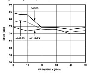
Figure 13. In-Band SFDR vs.  $f_{OUT} @ f_{DATA} = 160 \text{ MSPS}$
