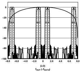
Figure 88. 8× Interpolation, Complex f<sub>DAC</sub>/8 Modulation
