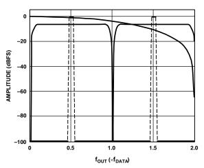
Figure 65.  $2 \times$  Interpolation, Modulation =  $f_{DAC}/4$
