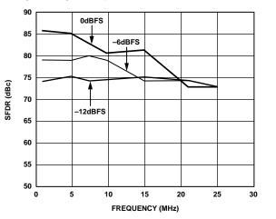
Figure 7. In-Band SFDR vs.  $f_{OUT} @ f_{DATA} = 65 \text{ MSPS}$
