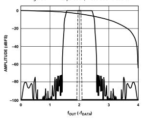
Figure 68. 4x Interpolation, Modulation =  $f_{DAC}/2$
