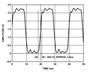
Figure 53. DATACLK Driver Capability into 330  $\,\Omega$  at 50 MHz
