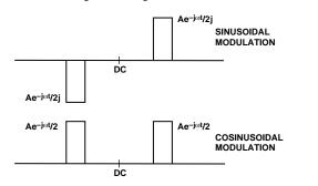
Figure 58. Baseband Signal, Amplitude Modulated with Sine and Cosine Carriers
