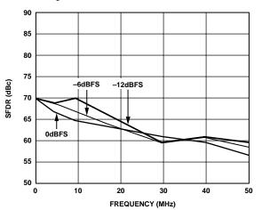
Figure 14. Out-of-Band SFDR vs.  $f_{OUT} @ f_{DATA} = 160 \text{ MSPS}$
