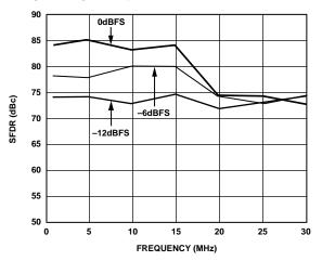
Figure 10. In-Band SFDR vs.  $f_{OUT} @ f_{DATA} = 78 \text{ MSPS}$
