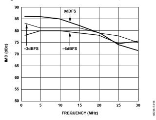
Figure 16. Third-Order IMD Products vs. Two-Tone  $f_{OUT} @ f_{DATA} = 78 \text{ MSPS}$
