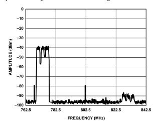
Figure 100. AD9777/AD8345 Synthesizing a Three-Carrier WCDMA Signal at an LO of 800 MHz
