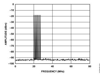
Figure 31. Eight-Tone IMD Performance,  $f_{DATA} = 160$  MSPS, Interpolation = 8x
