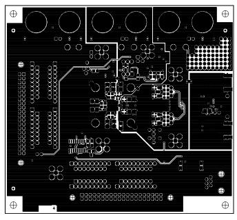
Figure 114. AD9777 Evaluation Board Layout, Layer Four (Bottom)
