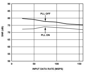
Figure 22. SNR vs. Data Rate for  $f_{OUT} = 5$  MHz
