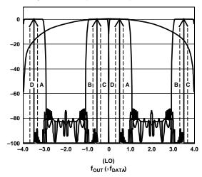
Figure 87.  $4 \times$  Interpolation, Complex  $f_{DAC}/8$  Modulation
