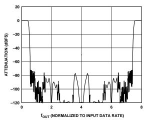
Figure 4.  $8 \times$  Interpolating Filter Response
