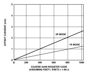
Figure 41. DAC Output Offset Current
