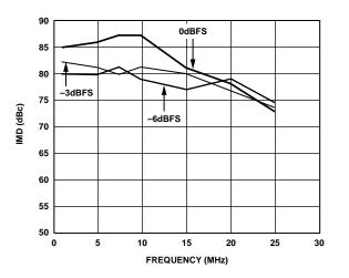
Figure 15. Third-Order IMD Products vs. Two-Tone fout @ f<sub>DATA</sub> = 65 MSPS
