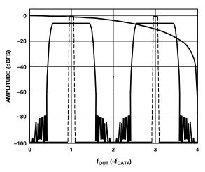
Figure 69. 4x Interpolation, Modulation =  $f_{DAC}/4$
