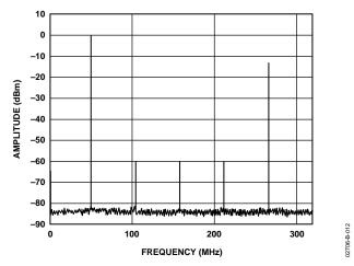
Figure 12. Single-Tone Spectrum @  $f_{DATA} = 160$  MSPS with  $f_{OUT} = f_{DATA}/3$
