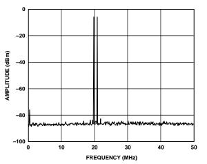
Figure 25. Two-Tone IMD Performance,  $f_{DATA} = 150$  MSPS, No Interpolation
