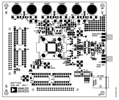
Figure 109. AD9777 Evaluation Board Components, Top Side
