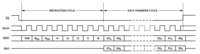
Figure 33. Serial Register Interface Timing MSB First
