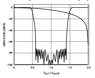
Figure 63. 2× Interpolation, Modulation = Disabled
