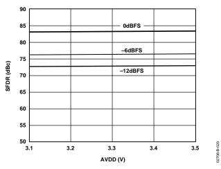
Figure 20. SFDR vs. AVDD  $f_{OUT} = 10 \text{ MHz}$ ,  $f_{DAC} = 320 \text{ MSPS}$ ,  $f_{DATA} = 160 \text{ MSPS}$
