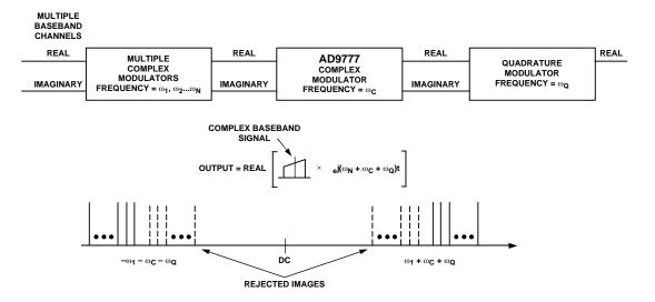
Figure 82. Image Rejection with Multicarrier Signals
