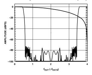
Figure 67. 4x Interpolation, Modulation Disabled
