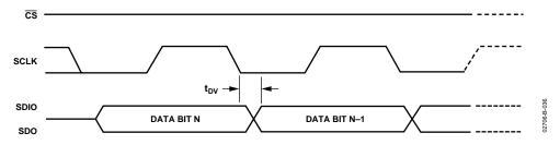
Figure 36. Timing Diagram for Register Read from AD9777
