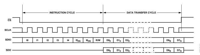
Figure 34. Serial Register Interface Timing LSB First
