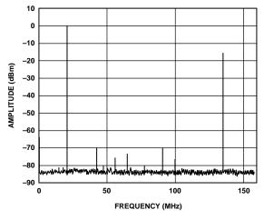
Figure 9. Single-Tone Spectrum @  $f_{DATA} = 78$  MSPS with  $f_{OUT} = f_{DATA}/3$
