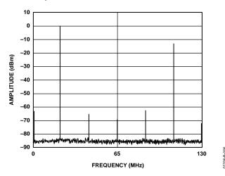
Figure 6. Single-Tone Spectrum @  $f_{DATA} = 65$  MSPS with  $f_{OUT} = f_{DATA}/3$
