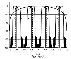
Figure 84.  $4 \times$  Interpolation, Complex  $f_{DAC}/4$  Modulation
